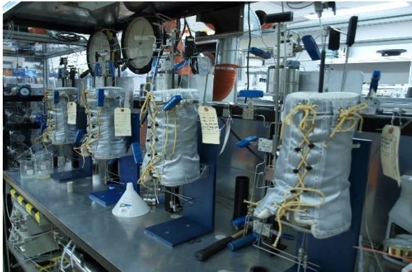
Figure 1: The steady state permeability apparatus used in this example has the capacity to measure permeability on four 1" Ø core plugs simultaneously.
