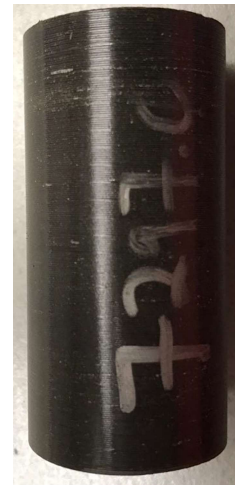
Figure 3: Vertical plug for geomechanical testing created using Premier’s technique for fragile core. In this example, perfect cylindrical samples were made from core that could not be plugged by conventional methods.
