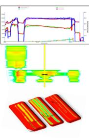
and enables computation of *in-situ* stresses when infill wells are completed alongside a depleted well. Now the calibrated model can be used to determine the optimum lateral landing, cluster spacing, number of clusters (based on effective fracture length), optimal fluid system (Hybrid vs. Crosslink vs. Slickwater), proppant type and proppant ramp and changes required to minimize asymmetry or changes to spacing.
